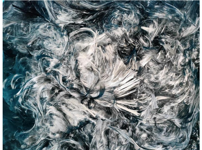
rCF – Image of the rCF obtained AFTER thermal treatment
