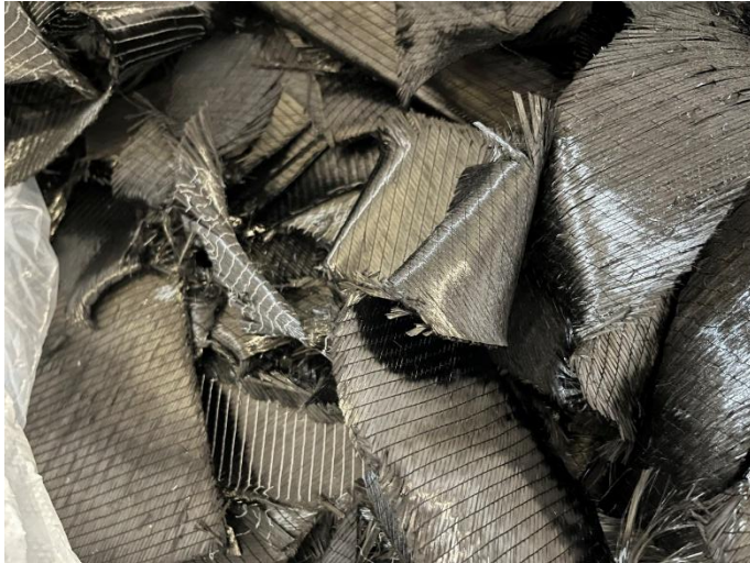
CFRP scrap – Image of CFRP BEFORE thermal treatment
