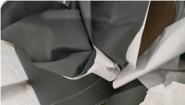
CFRP scrap – Image of CFRP BEFORE thermal treatment
